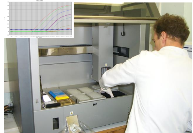
Robotic sample preparation for rRT-PCR
