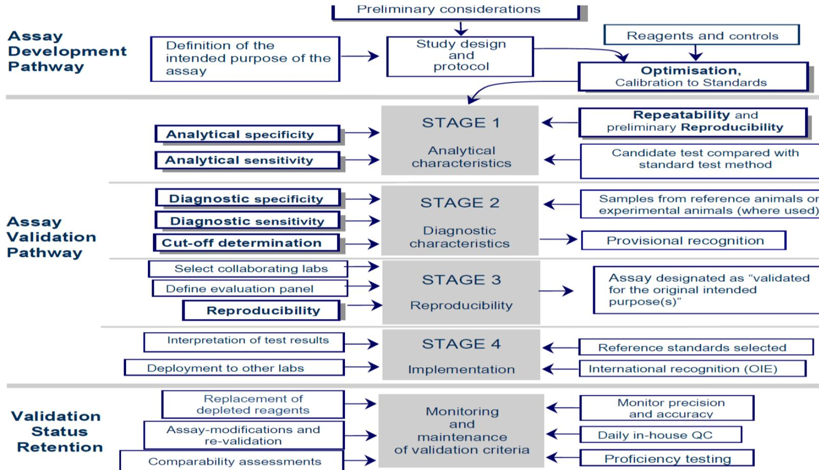
**Figure 1.** The assay development and validation pathways with assay validation criteria highlighted in bold typescript within shadowed boxes.
