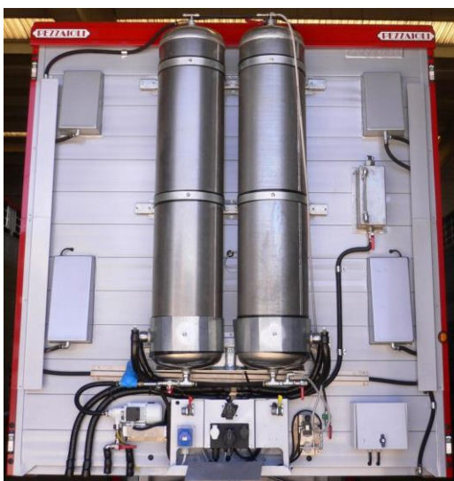
Image 46: Water tanks on the lorry for water supply of pigs (adapted from BTSF)
